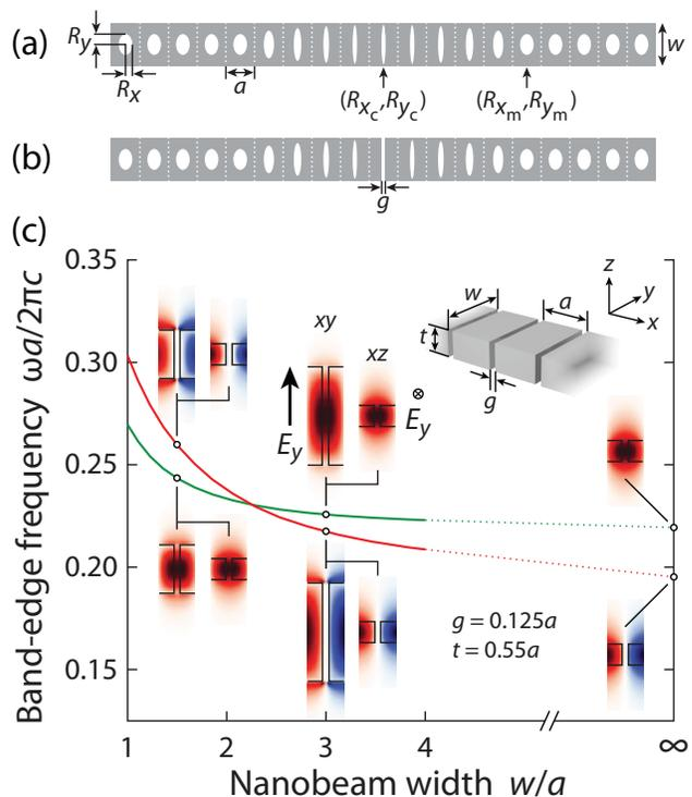
Fig. 1. (a) Schematic of donor-mode nanobeam cavity with elliptical holes. (b) Schematic of “split-beam” cavity with a rectangular gap defect at center. (c) “Gap unit cell” band-edge frequencies and electric field profiles for TE-like ( $y$ -odd,  $z$ -even) modes as a function of nanobeam width. For the mode profiles, the dominant  $E_y$  component is plotted for the  $xy$  and  $xz$  planes.
