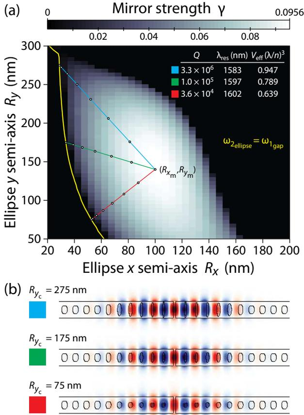
Fig. 3. (a) Mirror strength and resulting design parameters for three split-beam cavities;  $a$ ,  $t$ , and  $w$ , and the three  $(R_{x_c}, R_{y_c})$  values are as in Figure 2. The half-cavity tapered ellipse shapes are shown by open circles. (b) Mode profiles ( $E_y$ ,  $xy$  plane) of the three cavities in (a).
