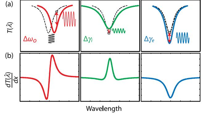
FIG. 2. Illustration of the effect of mechanical displacement on the optical response of a cavity with (left) dispersive, (center) dissipative intrinsic, and (right) dissipative external optomechanical coupling. (a) Change in the resonance line shape. (b) Amplitude of the optomechanically actuated signal.
