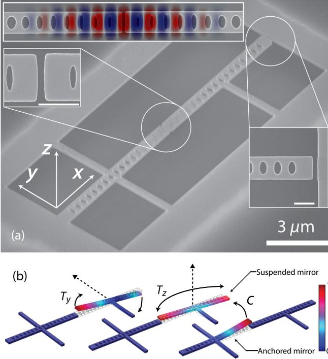
FIG. 1. (a) Scanning electron micrograph of a split-beam nanocavity. Top left inset: Top view of the nanocavity overlaid with the field distribution ( $E_y$ ) of the optical mode. Left inset: 60-nm-wide nanocavity central gap. Right inset: Gap separating the suspended nanobeam from the device layer. Inset scale bars: 500 nm. (b) Displacement fields of split-beam nanocavity mechanical modes of interest. Dotted arrows indicate the position and direction of torque for efficient actuation.
